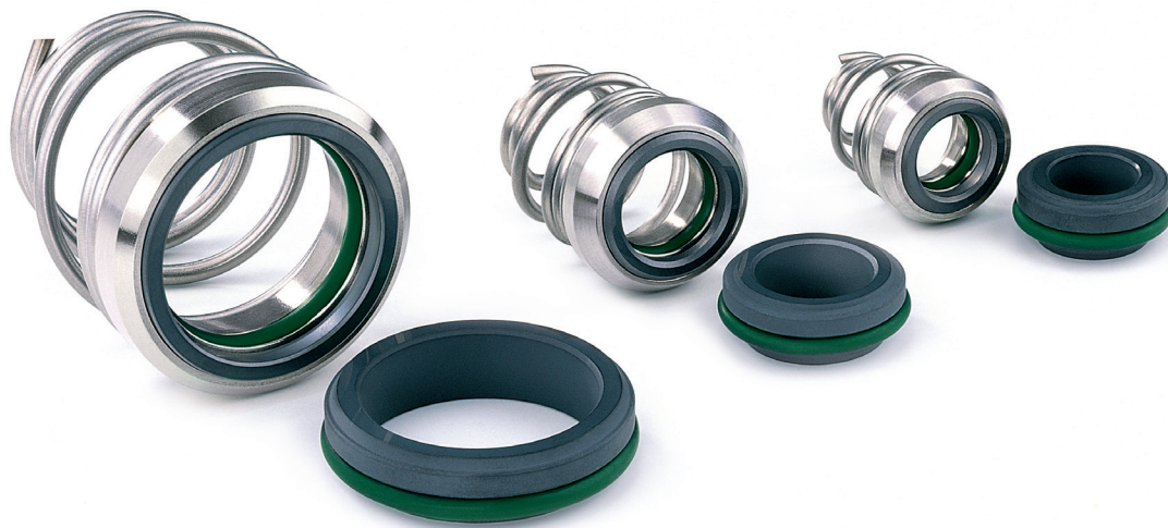
Type 33H , all material parts are in titanium including the self-driving spring. Shrunk-in SiC rotating ring and massive stationary SiC ring.
